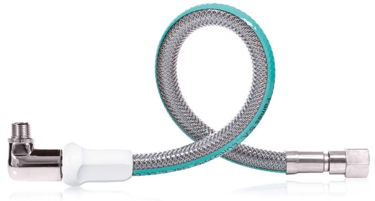
Gas coupler with metal elastic joint Nut of rotatable joint Rp 1/2" + valve. Minimum semi-diameter of multiplex flexion: R work 50 mm. MOP: 0,5 bar.
